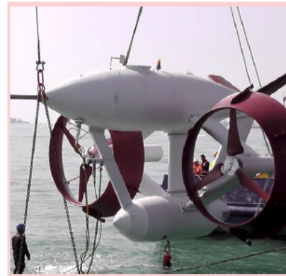
Pod-racer: the 20kW Ocean Kite prototype
