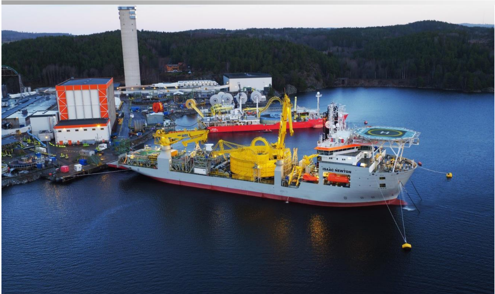
Norway – Loading of a 101 km Long Power Cable of 8,500 tonnes for the Marjan GOSP Project in Saudi Arabia - CLV Isaac Newton
