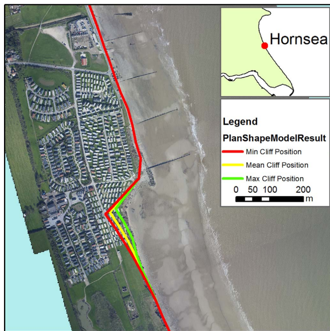
Fig. 16. Representation of the modelled probabilistic behaviour of the cliff at the southern end of the Hornsea defences throughout a ten-year period.
