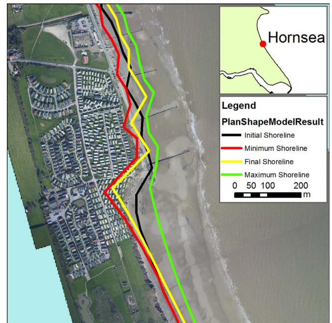
Fig. 15. Representation of the modelled probabilistic behaviour of the shoreline at the southern end of the Hornsea defences throughout a ten-year period.
